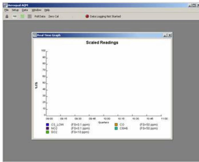
The Y-scale is given as percent full scale. The full scale reading is given beside the sensor name (eg CO<sub>2</sub> FS=2000 ppm) The Full scale can be changed for each sensor by clicking on 2000
