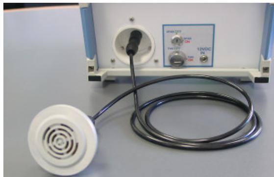
Extension cable for Temperature and Humidity sensor
