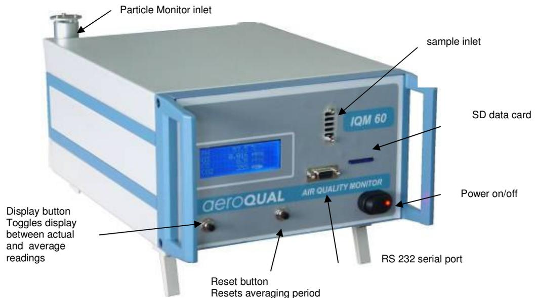
**NOTE 1.** Insert the data card by pressing in gently until the card latches in place. To remove the data card gently press inwards and then let go to release the latch. Always turn off the IQM 60 before removing or inserting the data card.
